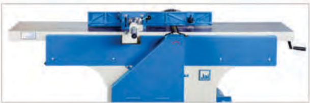
Infeed table longer than outfeed table for better accuracy & extra support
