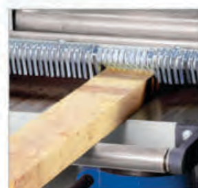
Anti kick-back system to avoid backsliding
