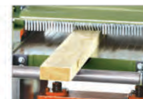
Anti kick-back System to avoid back sliding
