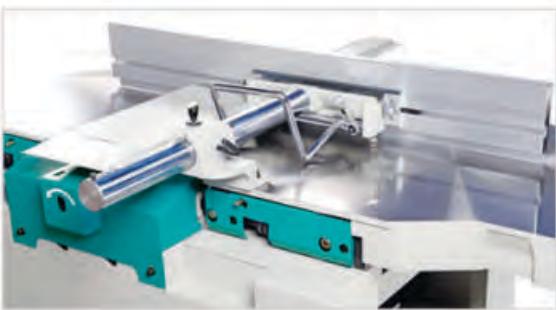
Manual movement of infeed surface table by means of parallelogram system. Ripfence fastened to a central support for an absolute rigidity.
